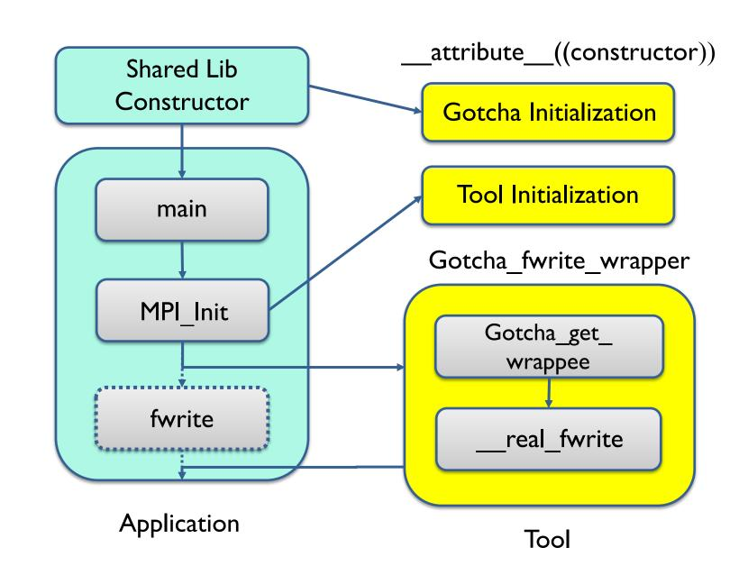
Fig 2. Modified control flow of an end-user application when using a Gotcha enabled tool with it.
